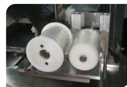
Ink residue pickup through pad cleaning system
