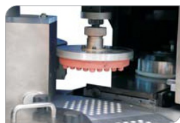
Enclosed Ink Pot & print transfer arrangement
