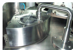
Quick drying arrangement using infrared heater after printing
